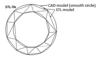
As shown in the figure, the shape of the object changes when the file is converted from a design file to a manufacturing-ready file in the 3D printing context. However, when the manufacturing-ready file is converted to a machine-instruction file, the overall object shape is unchanged; rather, the shape as depicted in the manufacturing-ready file is utilized exactly to provide precise instructions to the manufacturing device.
